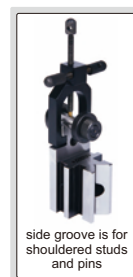
the adjustable screw can support the block and prevent tilting
