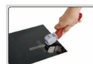
step 1: make grid cutting on surface
